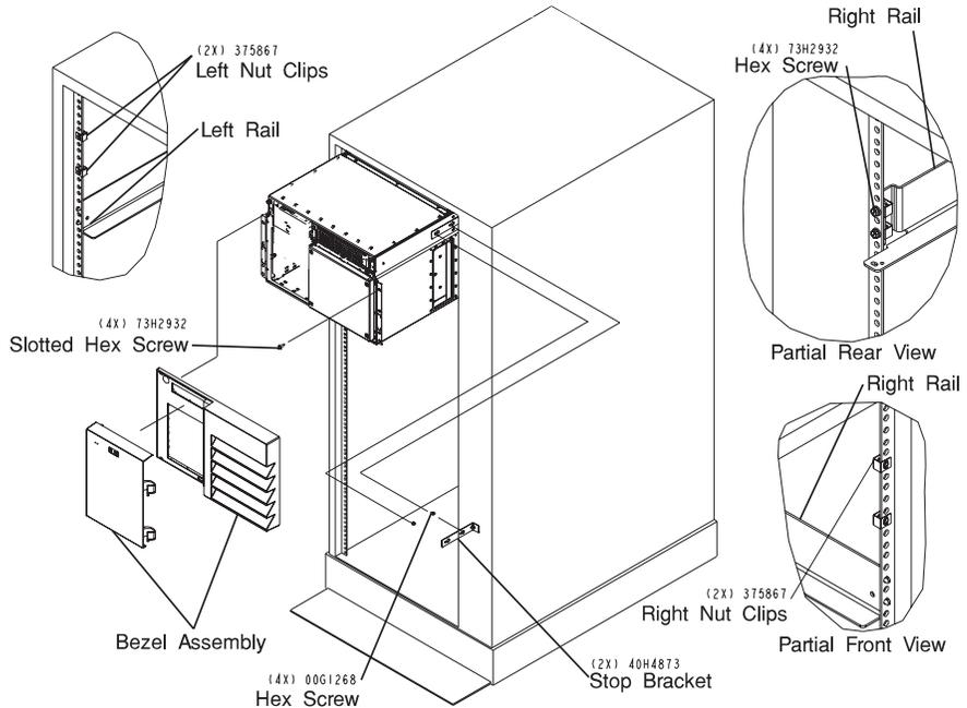
3. Lift the I/O Drawer onto the support rails, and slide it **slowly** into the rack until the first hexhead flange screw. Slip the angled end of each chassis stop bracket behind the rack frame and position the slotted clearance holes over the hexhead flange screws. Tighten the hexhead flange screws securely.
