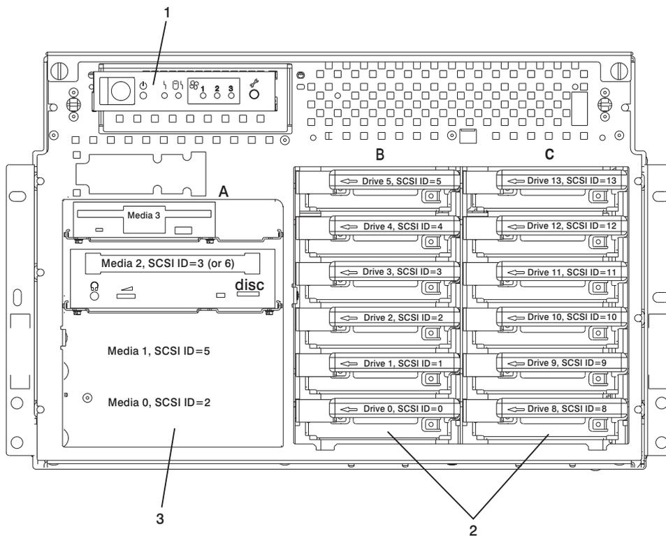
**Note:** The SCSI IDs shown for Media Bay A indicate how installed devices will be set when shipped from the factory.
