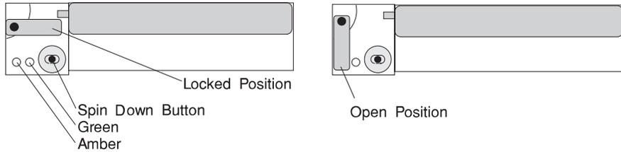
The following table explains the meaning of the green and amber status lights and spin down button on a SCSI disk drive.
