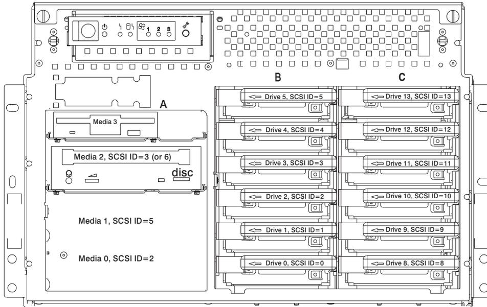
**Note:** The SCSI IDs shown for Media Bay A indicate how installed devices will be set when shipped from the factory.
