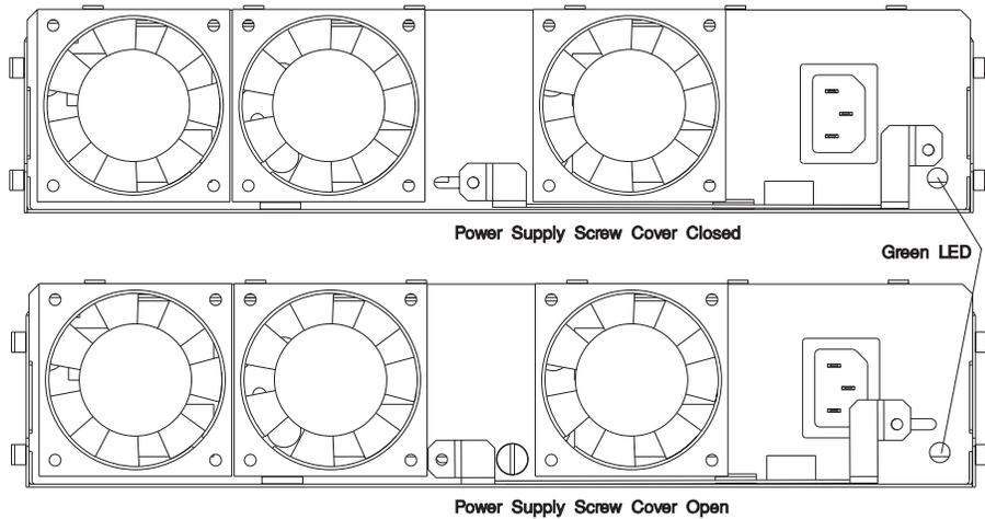
8. Loosen the screw until the power supply can be pulled out.
