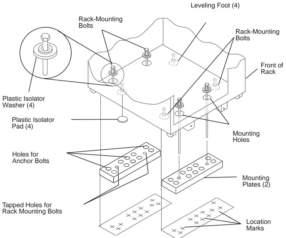
20. Tighten the four rack-mounting bolts into the two mounting plates.
