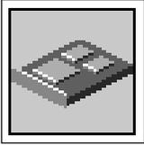
The **Config** icon allows you to configure network adapters which are recognized by the system as requiring setup. Selecting the Config icon presents a list of the adapters requiring configuration. Use the arrow keys to highlight an adapter, press the spacebar to select the adapter, then highlight the **OK** icon and press the Enter key.
