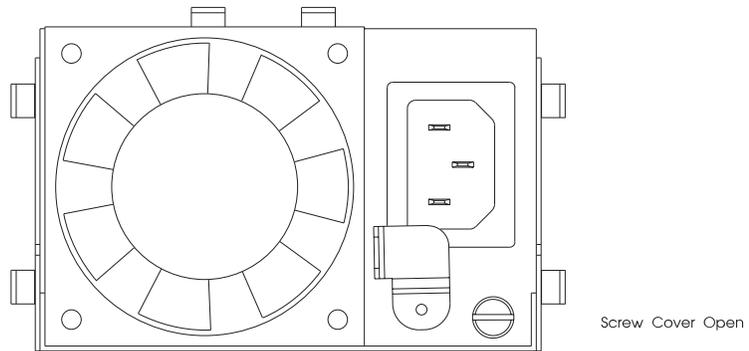
5. Plug the power cord into the power supply.
