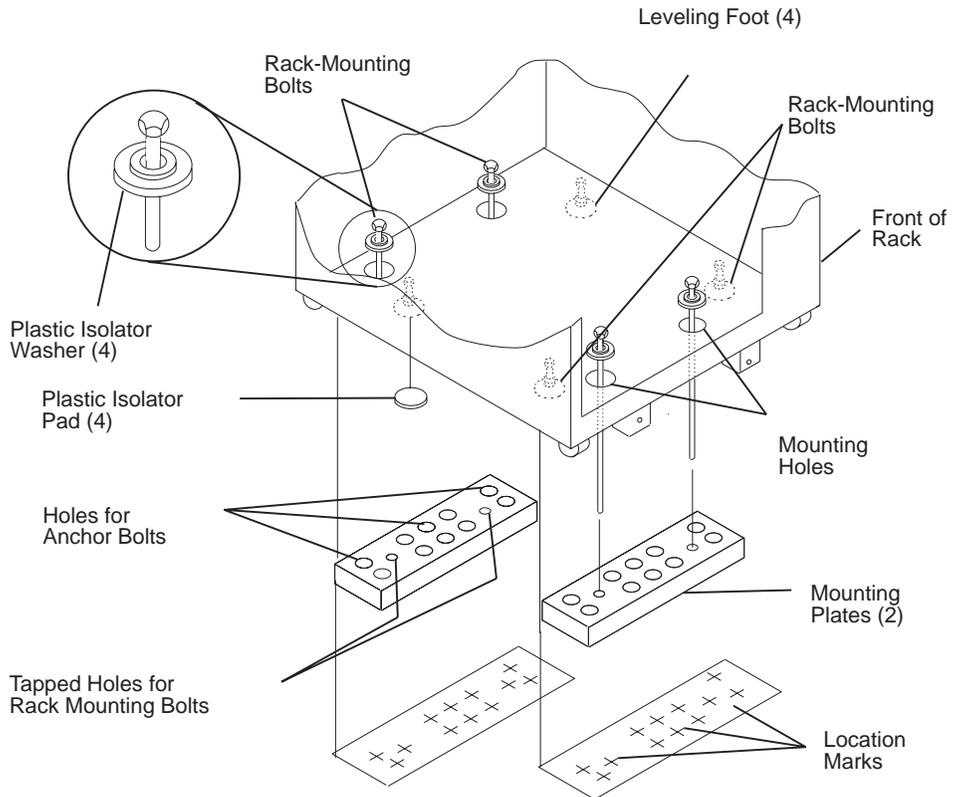
17. Tighten the four rack-mounting bolts into the two mounting plates.
