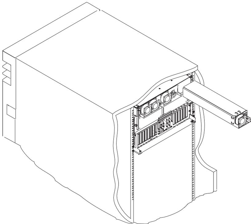
7. To remove the 3/4 power supply, slide the screw cover to the left to the open position to access the power supply screw.
