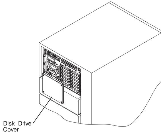
**Attention:** Physically removing a hot swap drive from the I/O Drawer before it has been removed from the system configuration, may cause unrecoverable data corruption.
