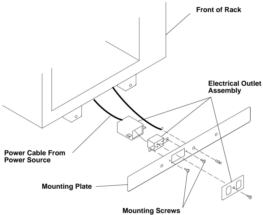
2. Place the ground cable lug through the mounting hole of the mounting plate.
