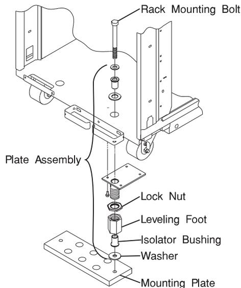
2. Place the mounting plates, front and rear, (note they are different) in the approximate mounting position under the System Rack.
