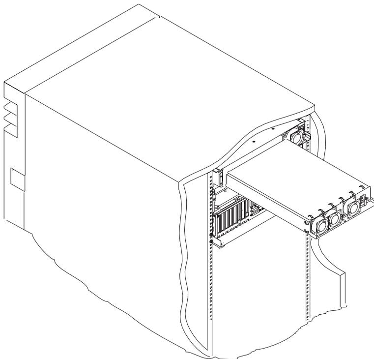
8. Tighten the screw until the power supply is drawn in tight.
