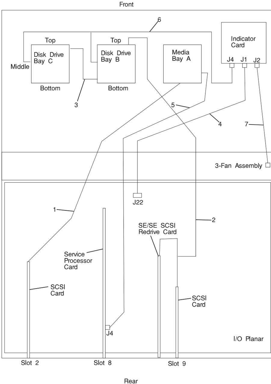
**Note:** The SCSI card may be installed in slot 9 or 13. The SP System Attachment PCI adapter must be installed in slot 10.
