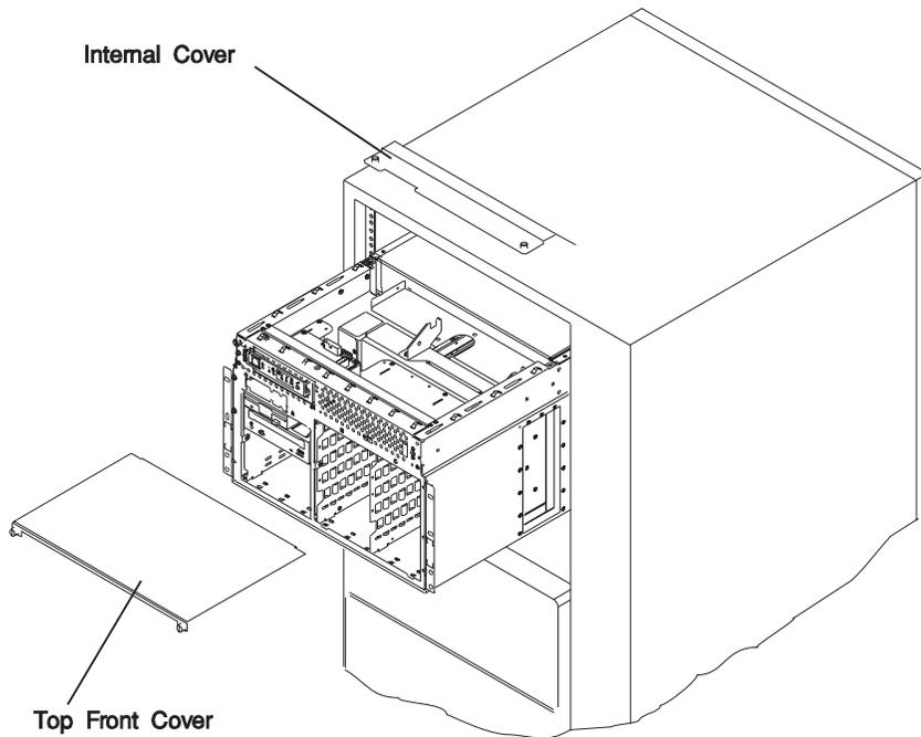
4. Remove the internal cover by loosening the two thumbscrews.
