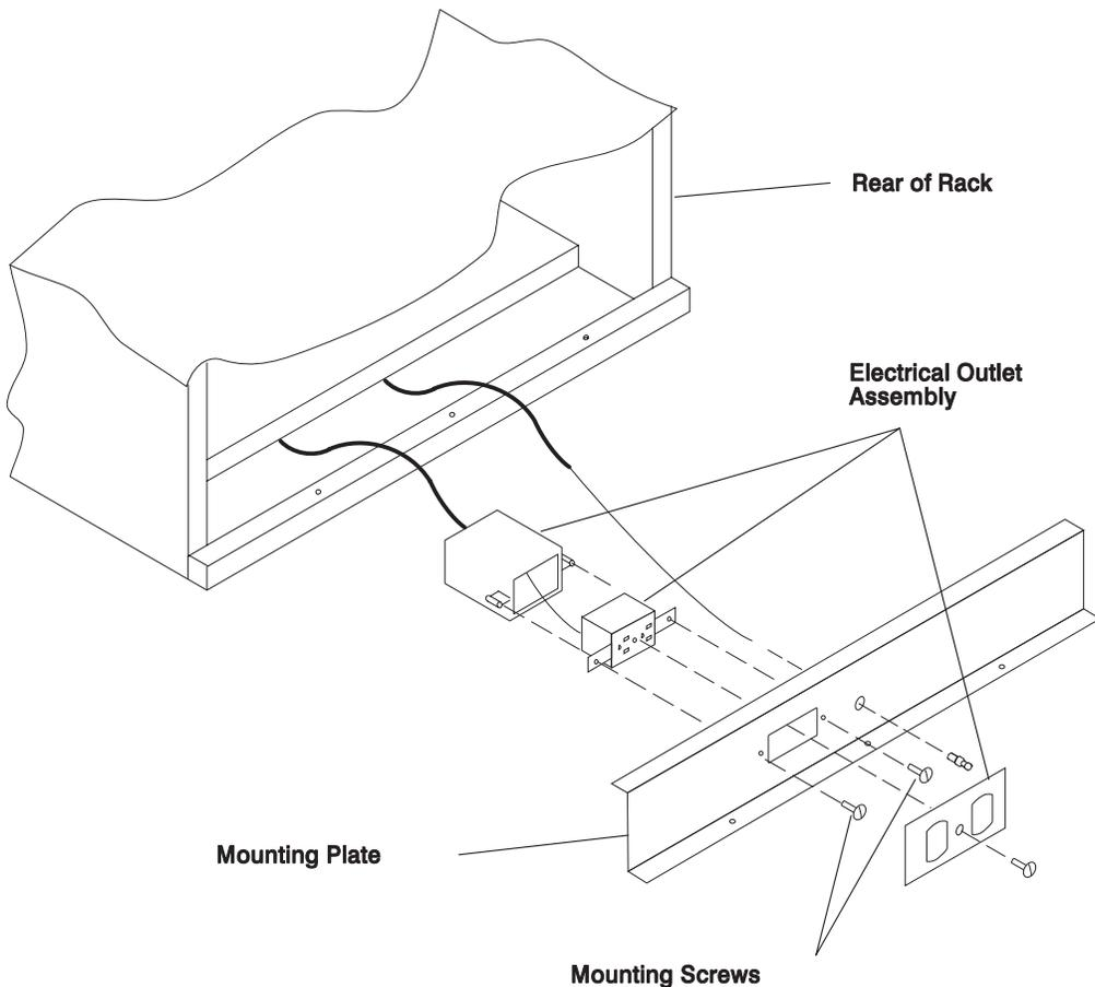
3. Place the ground cable lug through the mounting hole of the mounting plate.
