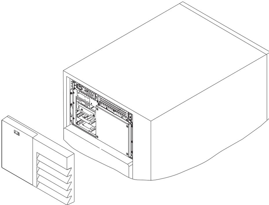
2. Remove the screws that hold the disk drive cover to the drawer and remove the disk drive cover from the drawer, storing it in a safe place.
