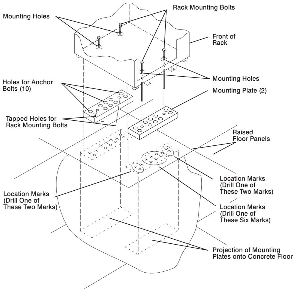
13. Place the two mounting plates on the locations indicated on the marked raised-floor panel.
