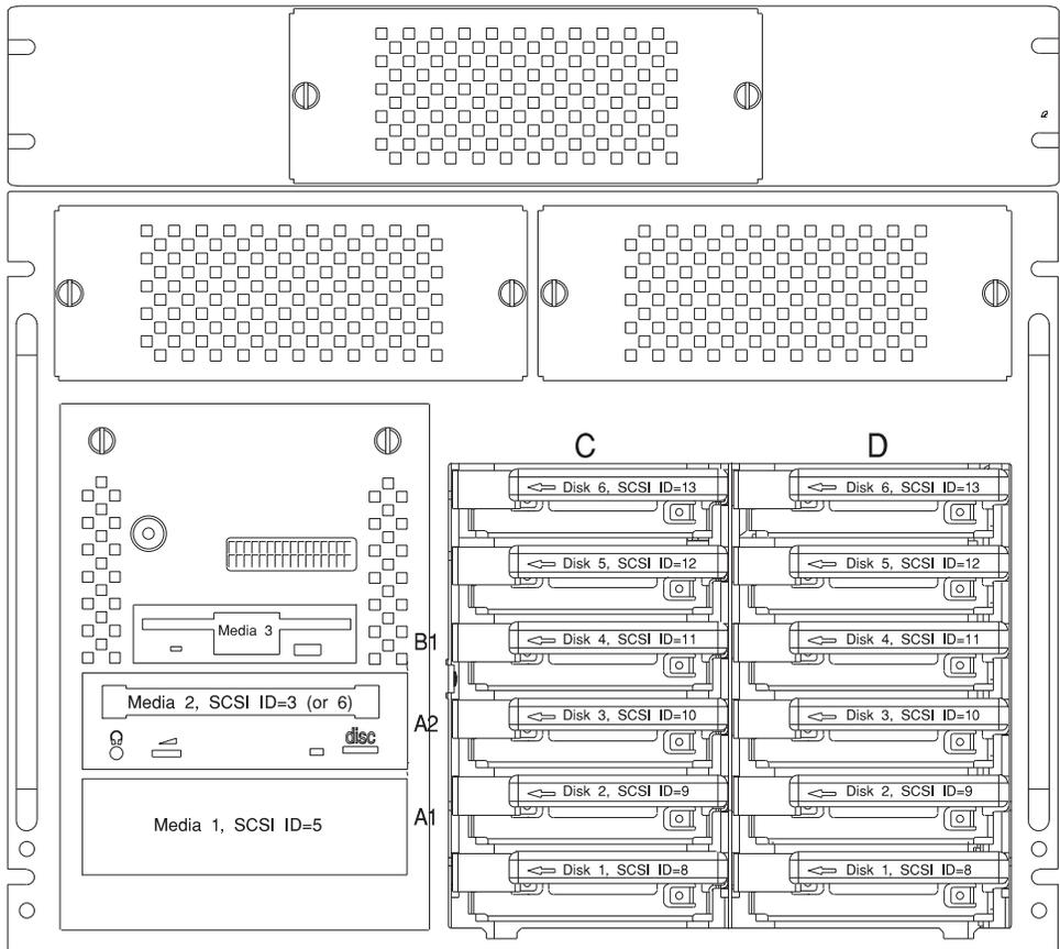
**Note:** The SCSI IDs shown for Media Bay indicate how installed devices will be set when shipped from the factory.
