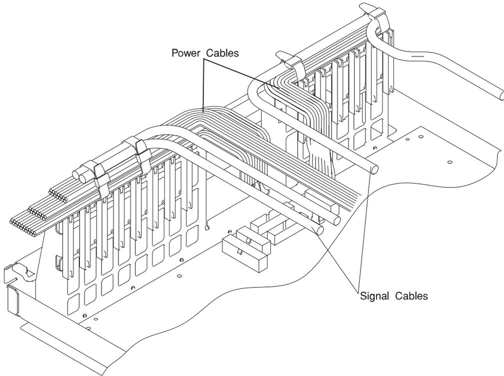
**Attention:** Take care to route power and signal cables on the top of the I/O adapter support. Retain the cables with unlocking wire ties as shown. This keeps the air entry cutouts in the drawer open and helps prevent adapters from overheating.
