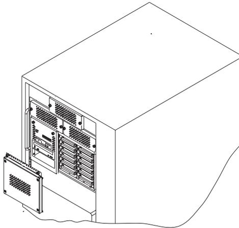
3. Each hot swap disk drive you plan to replace must have the hot swap SCSI disk drive carrier attached.
