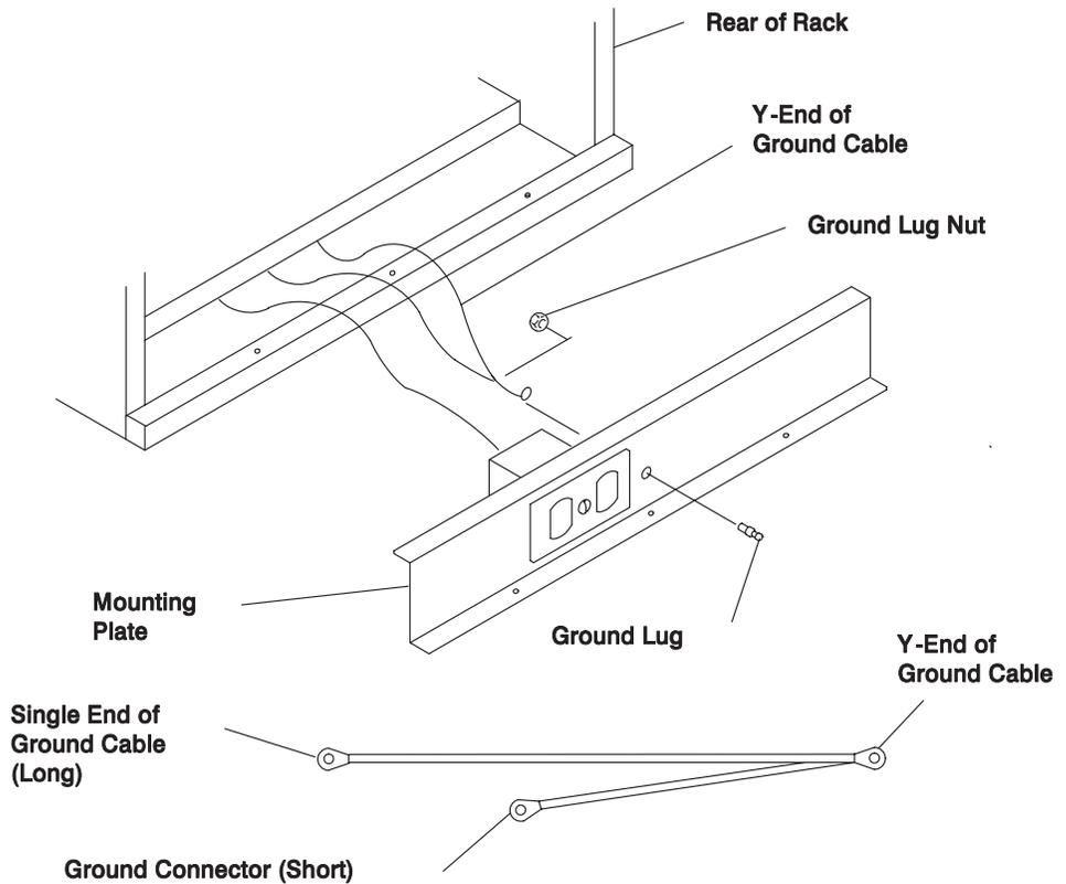
5. Attach the mounting plate to the rack by installing and tightening the three mounting screws.
