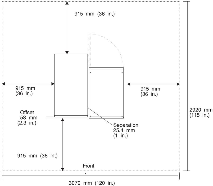
**Note:** Rack units are large and heavy and are not easily moved. Because maintenance activities require access at both the front and back, extra room needs to be allowed. The footprint shows the radius of the swinging doors on the Input/Output Rack. The illustrations show the minimum space required.
