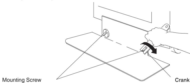
9. Hang the crank and tightening rod on the bracket near the bottom of the right wall inside the back of the rack.
