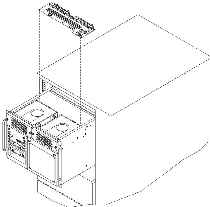
**Replacement:** Attach the new power distribution board to the bracket, and replace in reverse order.
