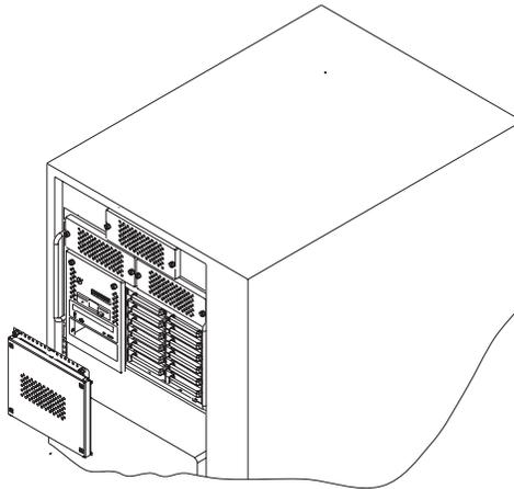
**Attention:** Physically removing a hot swap drive from the 10 EIA-Unit I/O Drawer before it has been removed from the system configuration, may cause unrecoverable data corruption.
