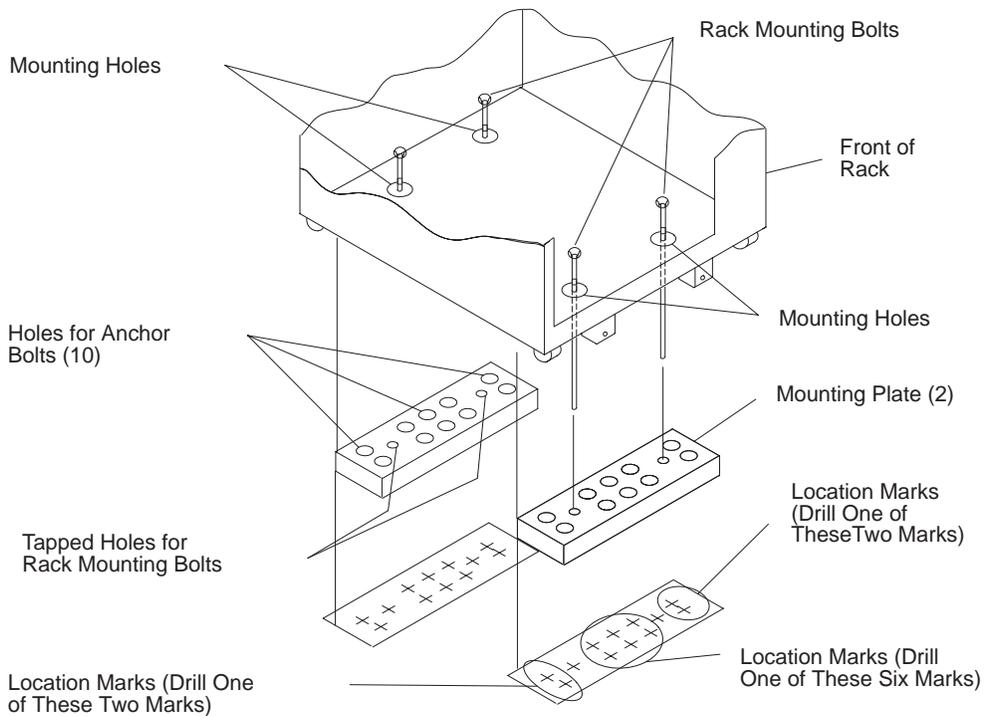
10. Drill one hole in each group of anchor bolt location marks as indicated on the marked floor.
