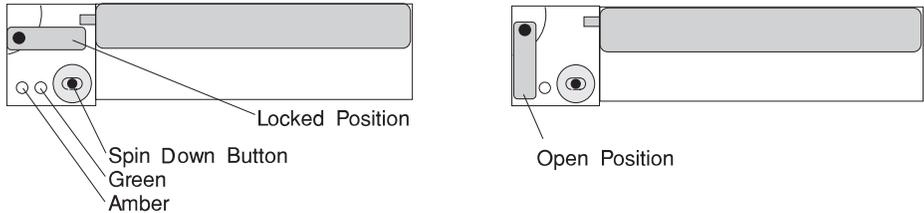
The following table explains the meaning of the green and amber status lights and spin down button on a SCSI disk drive.
