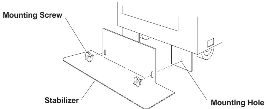
8. Use the crank supplied with the system unit to alternately tighten the mounting screws until they are firmly seated.
