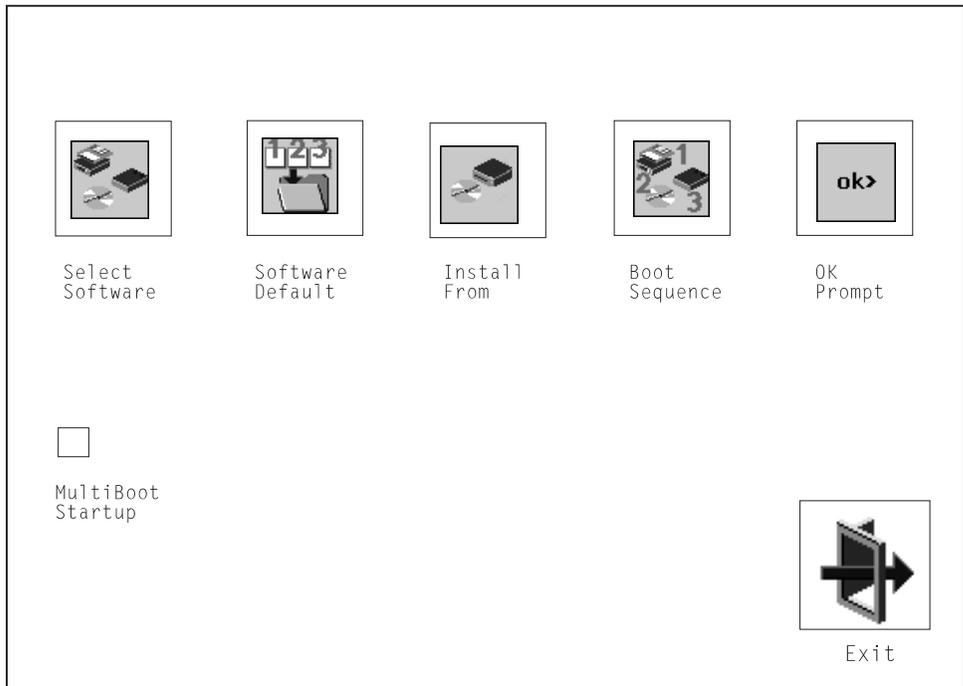
**Select Software:** If supported by the operating system, shows the names of the operating system installed. This option may not be supported by all operating systems.
