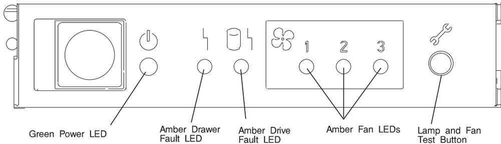
External indicators on the front indicator panel indicate status for functions in the I/O Drawer and they are visible with the rack door open. They are:
