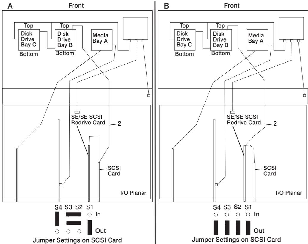
Figure A shows SCSI disk drive bay cabling and SCSI card jumper settings when using cable FRU PN 93H2456
