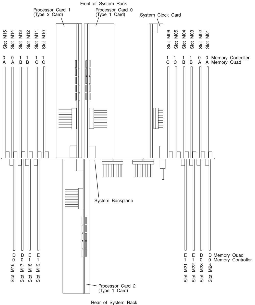
R1 Memory Cards are the primary memory cards used in the S70 and S7A systems. All memory cards are installed in four card functional units called quads. The quads must be composed of the four cards of the same type. The complete set of four cards must be properly installed in the proper card slots for the newly installed memory to work. See the figure on page 1-27 for the location of the card slots that are in each quad.
