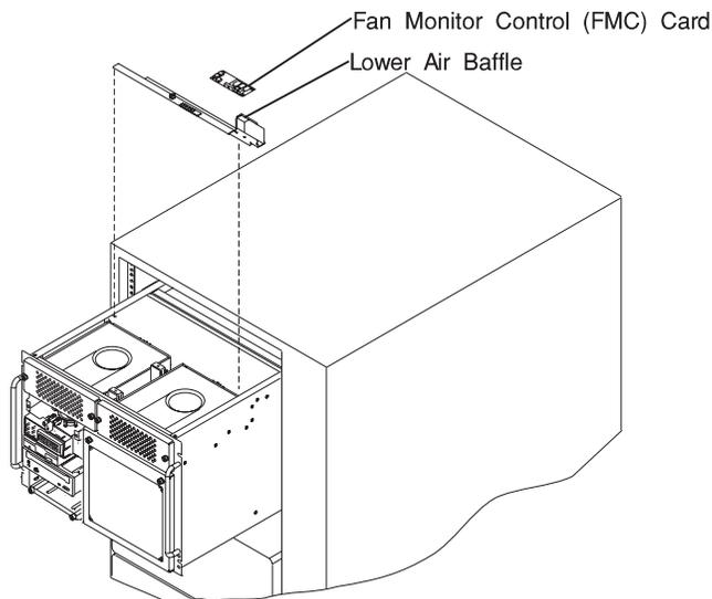
6. Remove the screws from the fan monitor control card and remove the card from the lower air baffle.
