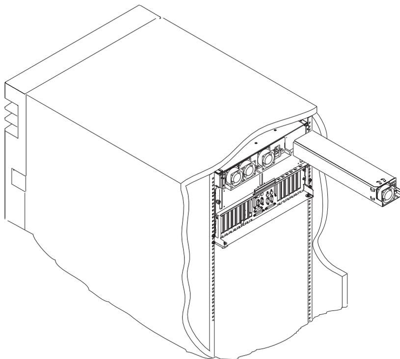
3. Tighten the screw until the power supply is drawn in tight.
