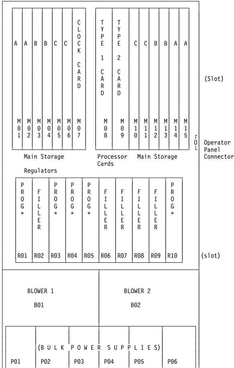
\* The S70 is manufactured with programmable regulators in positions R01, R03, and R10. The S7A is manufactured with programmable regulators in positions R03, R04, and R05. Filler cards are installed in any empty regulator positions.
