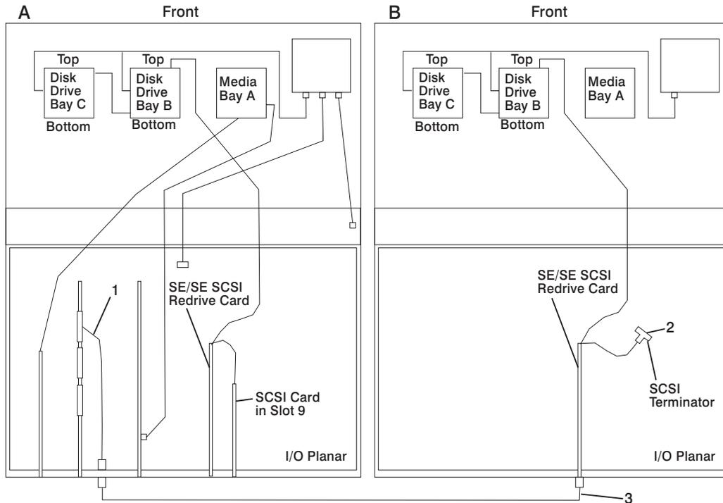
Figure A shows the primary I/O drawer with the disk drive bays connected to the SCSI card installed in slot 9. Figure B shows a secondary I/O drawer with the SCSI disk drive bays connected through an external cable to the SE/SE Redrive card. This external connection can be made between cards in the same drawer.
