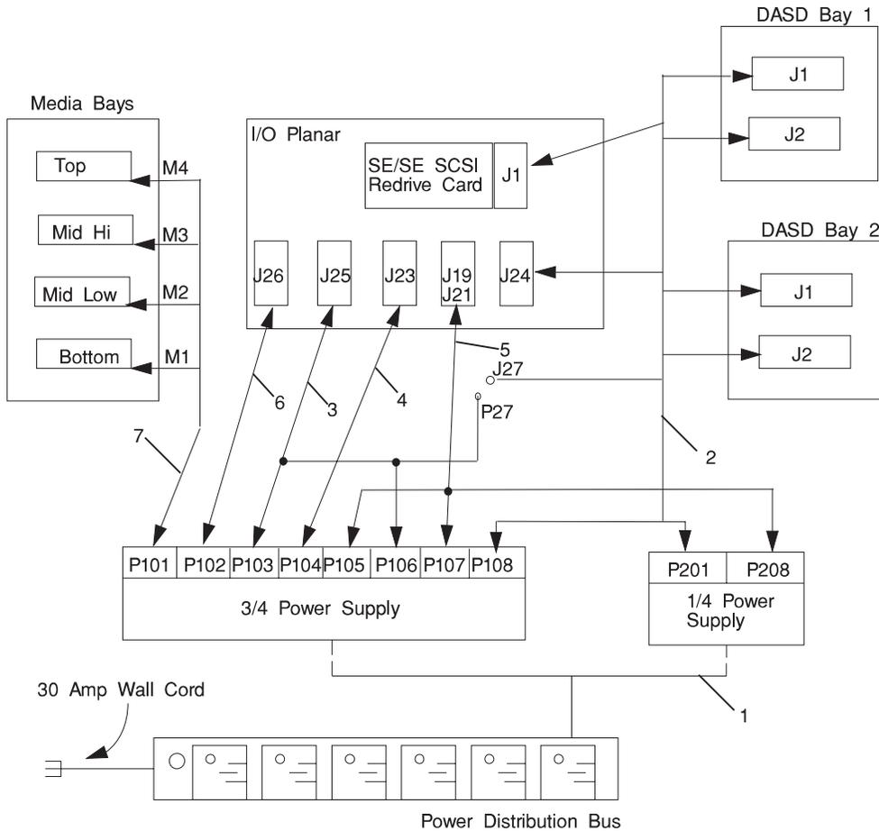
**Note:** The power distribution bus, and the Y-cable (index number 1) shown above are not used on -48 V dc systems. See “Input/Output Rack -48 Volt Power Distribution Assembly (2 of 2)” on page 10-62 for -48 V dc power distribution parts.
