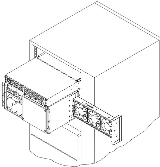
**Replacement:** Replace in reverse order. Ensure that the retained screws are properly engaged, as they draw the fan assembly into the fan connectors.
