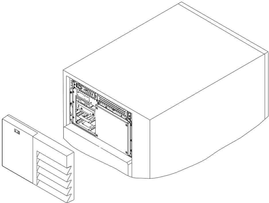
2. Loosen the screws that hold the disk drive cover to the drawer and remove the disk drive cover from the drawer, storing it in a safe place.
