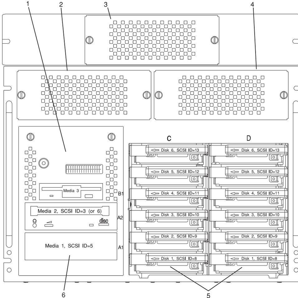
**Note:** The SCSI IDs shown for Media indicate how installed devices will be set when shipped from the factory.
