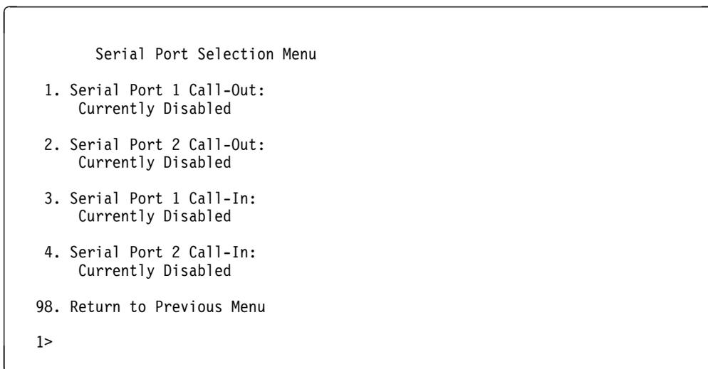
You may enable and/or disable the call-in and call-out functions of each serial port in any combination.
