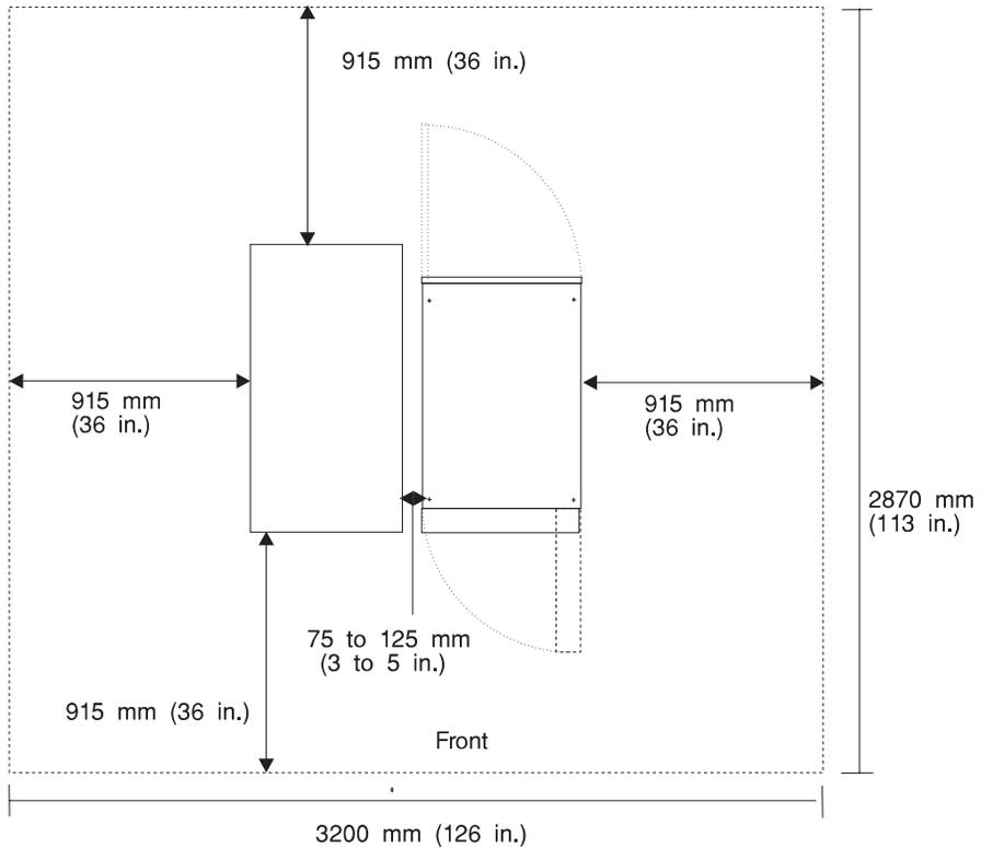
**Note:** Rack units are large and heavy and are not easily moved. Because maintenance activities require access at both the front and back, extra room needs to be allowed. The footprint shows the radius of the swinging doors on the I/O rack. The illustrations show the minimum space required.
