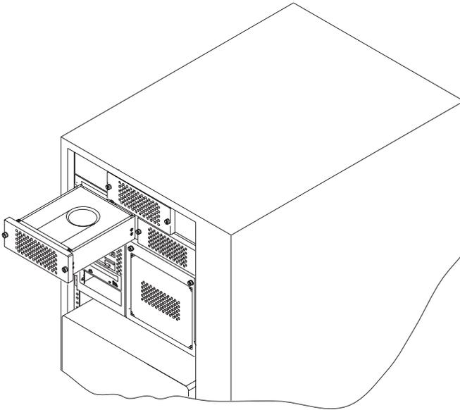
**Replacement:** Replace in reverse order. Ensure that the retained screws are properly engaged, as they draw the blower assembly into the blower connectors.
