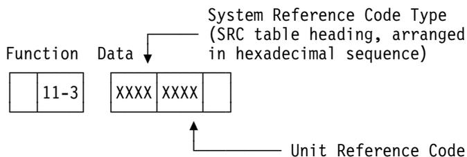
Figure 6-1. Determining the SRC and URC
