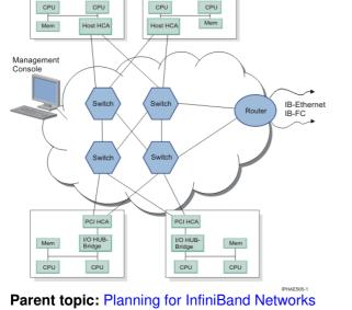
Figure 1. Servers configured in an InfiniBand (IB) network
