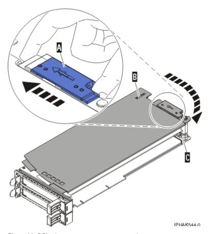
Figure 99. PCI adapter cassette cover removed
