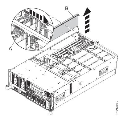
Figure 8. PCI adapter or filler plate removed from the rack-mounted system unit
