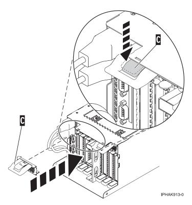
Figure 57. PCI adapter EMC shield in the closed position
