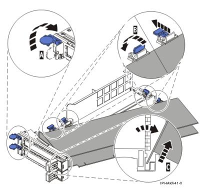
Figure 100. Adapter removed from the PCI adapter cassette
