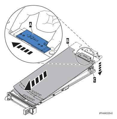
Figure 76. PCI adapter cassette cover replaced
