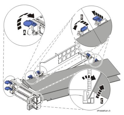
Figure 78. Adapter removed from the PCI adapter cassette
