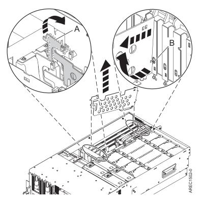
Figure 28. PCI-adapter divider removed from the system unit
