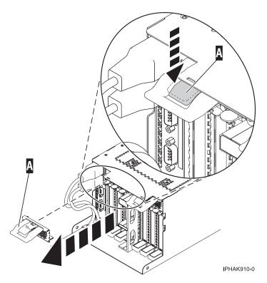
Figure 33. Remove the EMC shield
