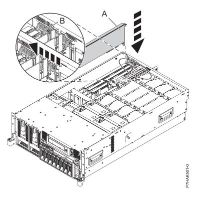
Figure 2. PCI adapter replaced in the rack-mounted system unit
