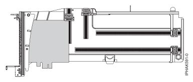
Figure 71. Side view of adapter in cassette
