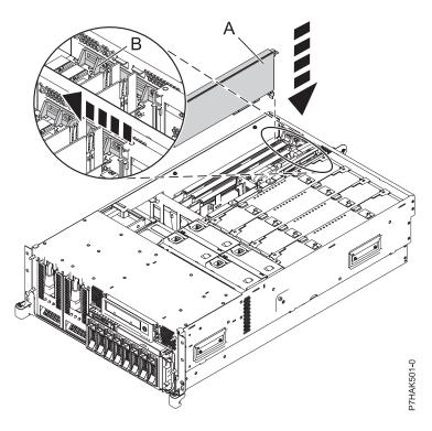
Figure 29. PCI adapter replaced in the rack-mounted system unit
