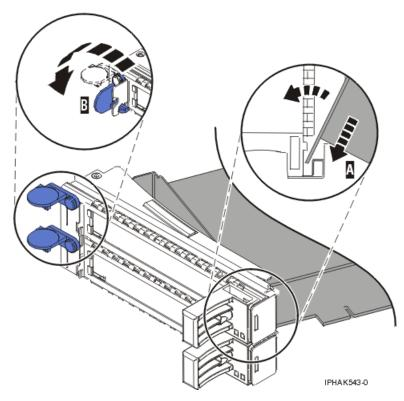
Figure 105. Adapter replaced in the PCI adapter cassette
