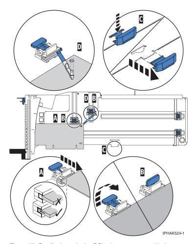
Figure 67. Small adapter in the PCI adapter cassette with the supports and the hookarm in place
