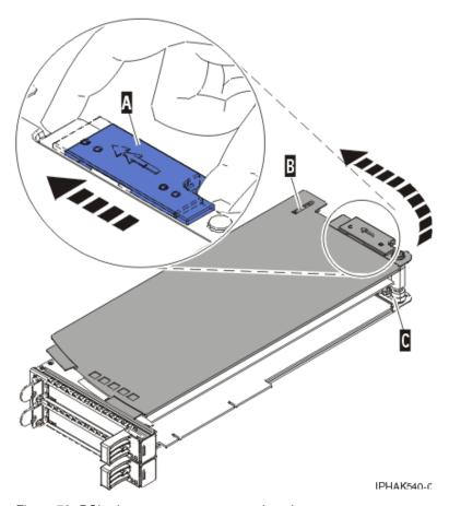
Figure 79. PCI adapter cassette cover replaced
