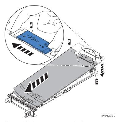
Figure 90. PCI adapter cassette cover replaced
