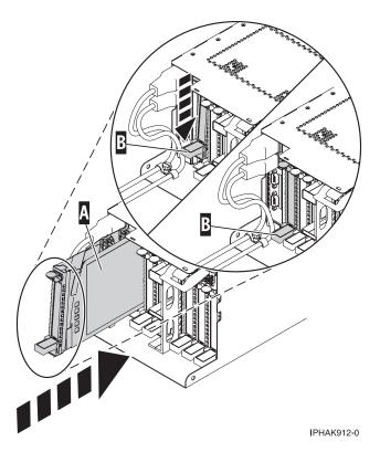
Figure 35. PCI adapter cassette installed in the system unit
