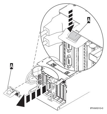
Figure 54. Remove the EMC shield
