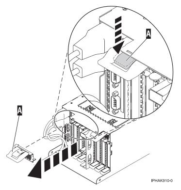
Figure 58. Remove the EMC shield
