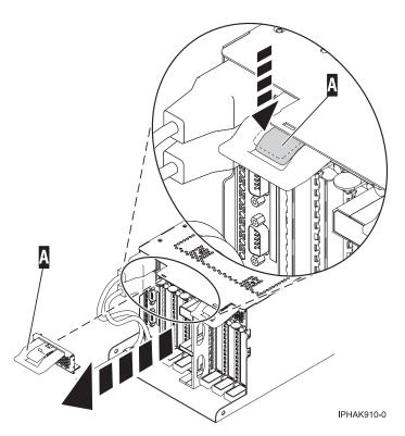
Figure 51. Remove the EMC shield
