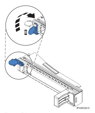
Figure 63. Tailstock clamp in the open position
