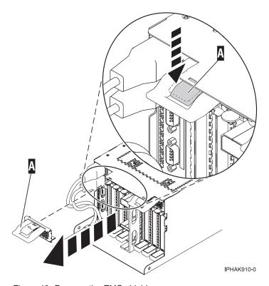
Figure 49. Remove the EMC shield
