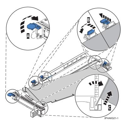
Figure 75. Adapter removed from the PCI adapter cassette
