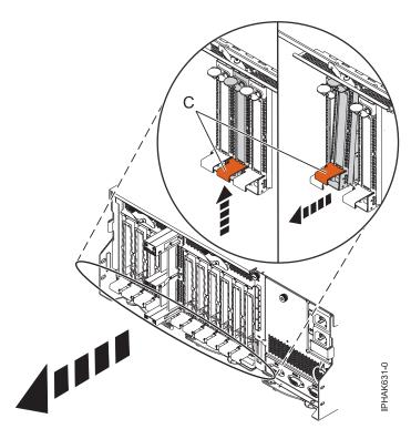
Figure 87. Removing a PCI adapter cassette
