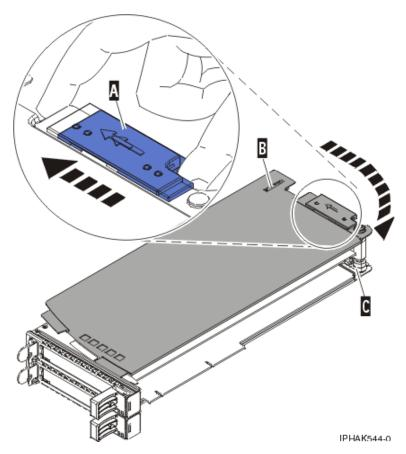
Figure 103. PCI adapter cassette cover removed
