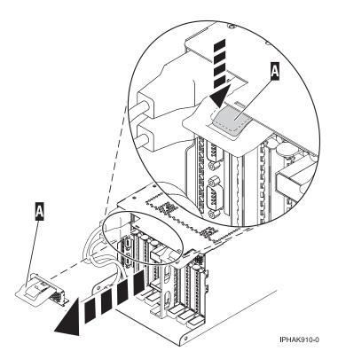
Figure 37. Remove the EMC shield
