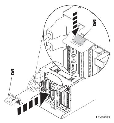
Figure 60. PCI adapter EMC shield in the closed position
