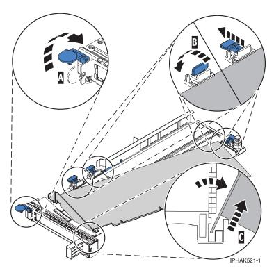
Figure 89. Adapter removed from the PCI adapter cassette
