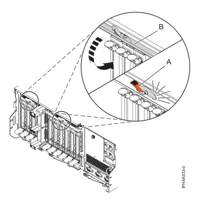
Figure 85. Closing the access door
