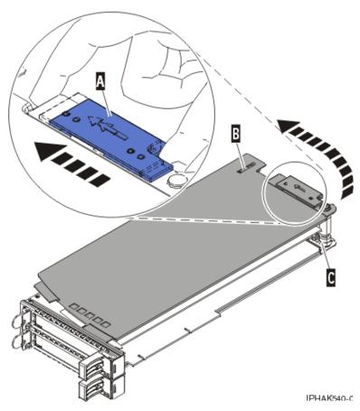
Figure 108. PCI adapter cassette cover replaced
