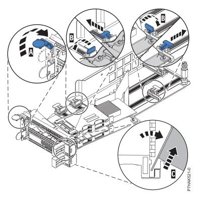
Figure 101. PCle RAID and SSD SAS adapter removed from the PCl adapter cassette
