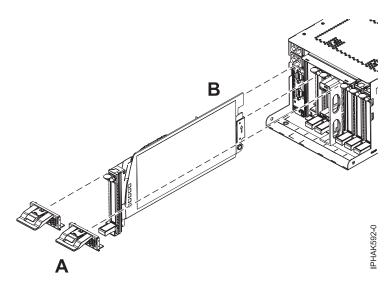
Figure 73. Replace the cassette and install the EMC grill
