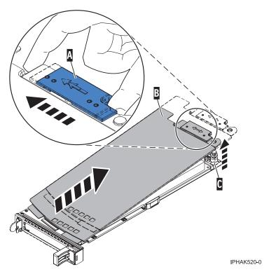
Figure 91. PCI adapter single-width cassette cover removed
