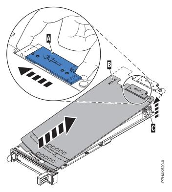
Figure 88. PCI adapter cassette cover removed
