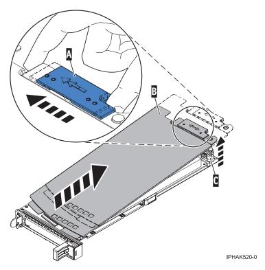
Figure 74. PCI adapter cassette cover removed
