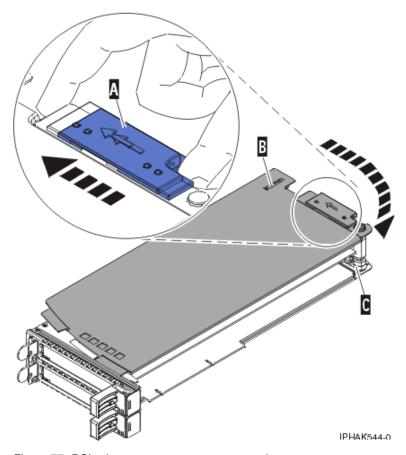
Figure 77. PCI adapter cassette cover removed
