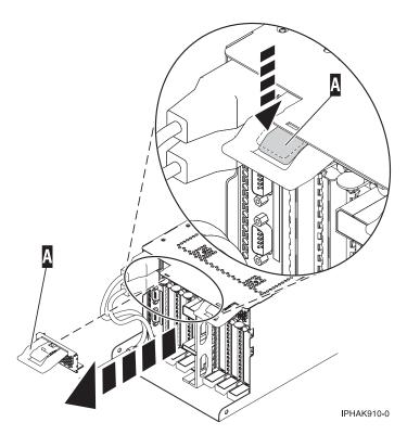
Figure 47. Remove the EMC shield
