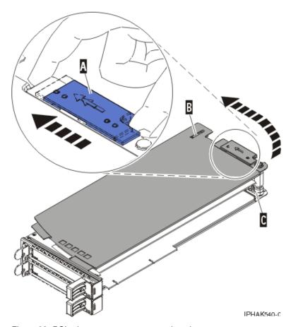
Figure 83. PCI adapter cassette cover replaced
