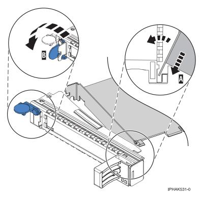
Figure 70. Placing the PCI adapter single-width cassette
