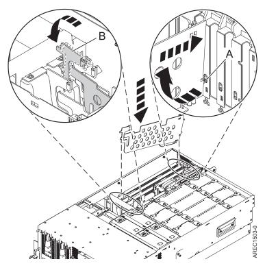
Figure 31. PCI-adapter divider replaced in the system unit
