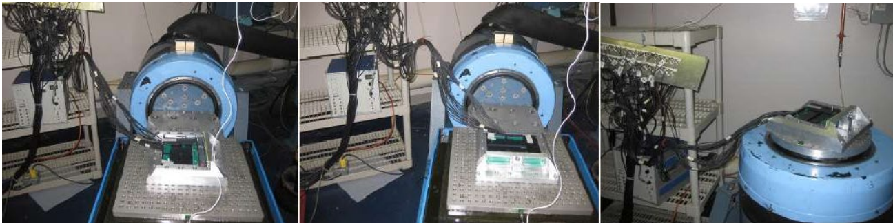
Figure 6: Vibration test set-up
