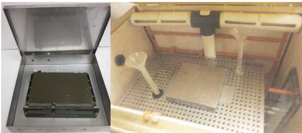
Figure 8: Salt Fog with SO 2 test set-up
