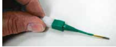
Plastic tool with contact in proper position.
