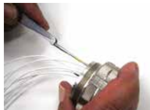
< Removal of contacts with metal tool.
