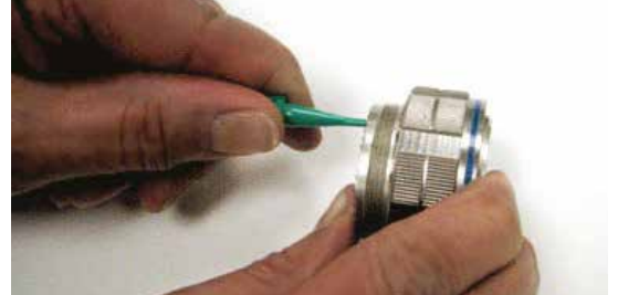
Plastic tool with contact in proper position.
