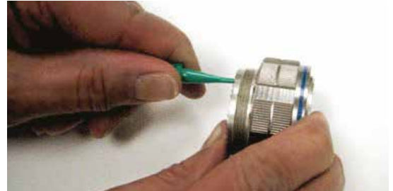
Plastic tool with contact in proper position.
