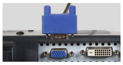
3 Make sure that your computer is turned off, then connect the other end of the video cable to the matching video port on the back of your computer.
