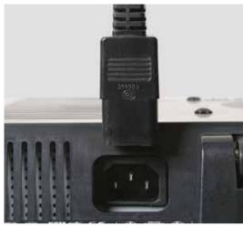
2 Plug the power cord into a correctly grounded power outlet. We recommend using a surge protector to protect your monitor from voltage spikes.
