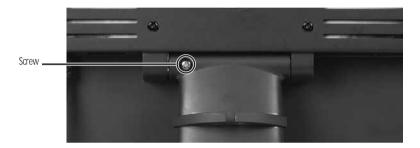
4 Remove the four small screws from the back of the LCD panel. Save the four screws.
