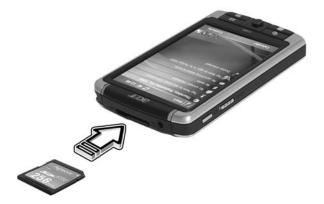
Push the card into the slot using your finger until you feel the card lock and hear an audible system sound. This indicates that the card is properly seated within the slot.
