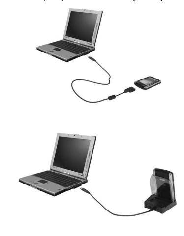
Plug the USB client connector into a USB port on your computer.
