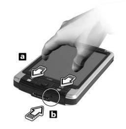
2. While holding the Today and Messaging buttons (**a**), using the tip of your stylus, lightly press the reset button inside the hole (**b**) on the bottom of your handheld.
