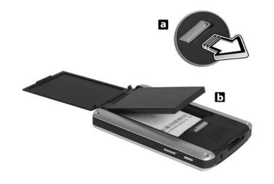
**NOTE:** To take the battery pack out, first unlock the battery access latch to open the battery cover, then pull the battery pack out of the bay.
