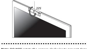
**Note:** DO NOT rotate the camera clockwise to prevent damage to the device.
