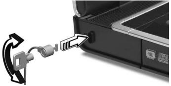
Wrap the computer security lock cable around an immovable object such as a table or handle of a locked drawer. Insert the lock into the notch and turn the key to secure the lock. Keyless models are also available.
